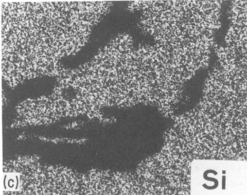
Figure 4 Back-scattered electron and X-ray micrographs of M_7C_3 solidification carbides in alloy T. The carbides appear enclosed in a tungsten-rich layer corresponding to the identified M_6C carbides.
